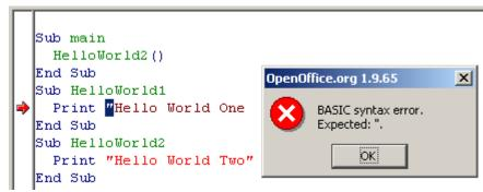
Figure 10. Click the Compile icon to find syntax errors such as a missing double quotation mark.
