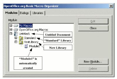
Figure 6. The TestLibrary contains one module named Module 1.
